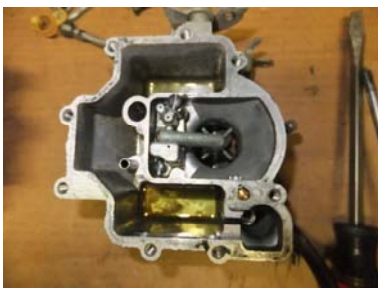
GREEN GOO FROM STOR- ING WITHOUT STABILIZING FUEL (high test from october!)
