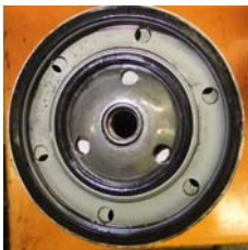
BAD OIL FILTER Restricted holes_plate shifted?
