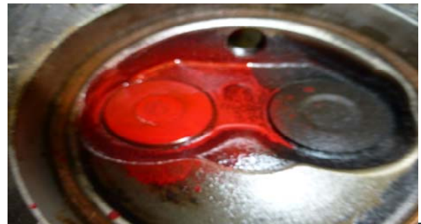
#5 exhaust valve seat sank just a little, and guide was leaking combustion into valve cover area. Hiss sound
