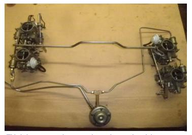
This is how to save time removing carbs etc when doing motor work. Remove as a unit. Just remember to check or replace base gaskets when reinstalling.
