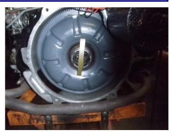
This shows a "tool" I made from an old diff sleeve and a piece of fiberglass to minimize wear on converter internals when running without a differential. I filled the sleeve with epoxy to seal it.
