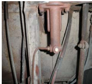
you never know what you will find (big pinch in the line) when you roll under an unknown vehicle (Phil's Loadside)
