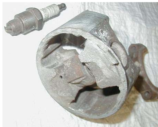
SOME RESULTS FROM DRIVING TOO FAR WITH NO FAN BELT
