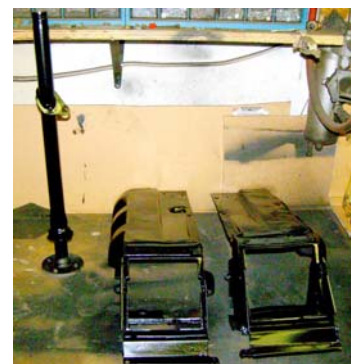
"reconditioned" lower shrouds and oil fill for the new "crampy" motor
