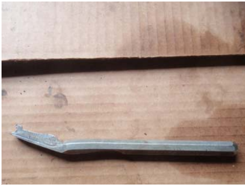
MY "MAGIC" TOOL FOR SEALS and-BEARINGS ON DIFFERENTIALS
