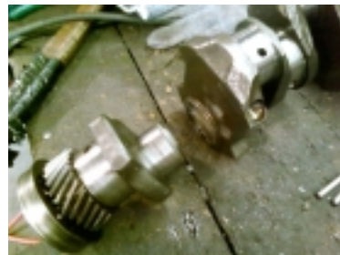
THIS IS A BROKEN CRANKSHAFT RESULTING FROM LACK OF A HARMONIC BALANCER, but it was on extreme conditions and lasted quite a while. Thanks to Warren for sharing his breakage pictures!
