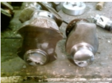
THIS IS A BROKEN CRANKSHAFT RESULTING FROM LACK OF A HARMONIC BALANCER, but it was on extreme conditions and lasted quite a while. Thanks to Warren for sharing his breakage pictures!
